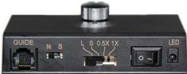
Figure 12. SkyGuider™ mount control board
